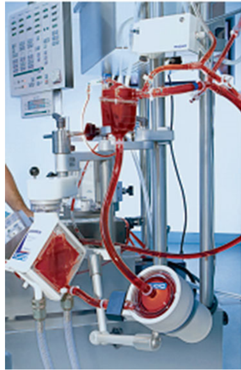
Fig. 11.2 Jostra Rotaflow ® is an example of a new generation of centrifugal pumps that eliminates the central drive shaft/bearing
