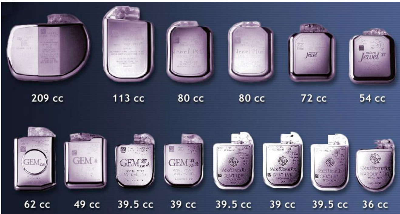
Fig. 30.18 The evolution of the implantable cardioverter defibrillator (ICD). Dramatic reductions in size have occurred, with simultaneous improvements in longevity, diagnostics, functionality, and memory
