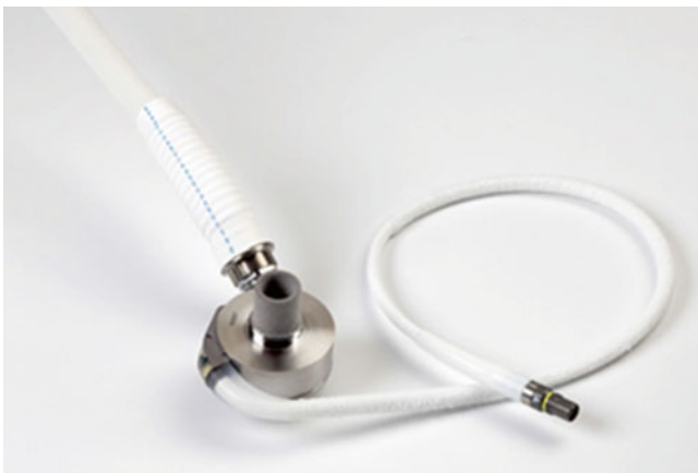
Fig. 11.6 Thoratec HeartMate III. This is a full-output centrifugal flow pump with a fully magnetically levitated rotor, which also allows the development of pulsatile flow. This near-physiological artificial pulse may have clinically important physiological benefits
