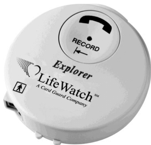
Fig. 19.14 A loop recorder with pacemaker and detection capabilities is shown. This model is manufactured by LifeWatch, Inc. (Rosemont, IL, USA)
