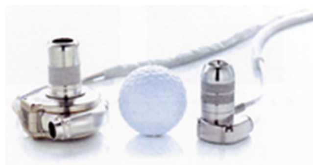
Fig. 11.5 HeartWare MVAD pump. This continuous axial-flow pump utilizes proprietary contactless impeller suspension technology and was designed to support a wide range of flows that enable full and partial support capability. Its small size and wide range of flows will likely enable support of smaller patients and those with right ventricular failure
