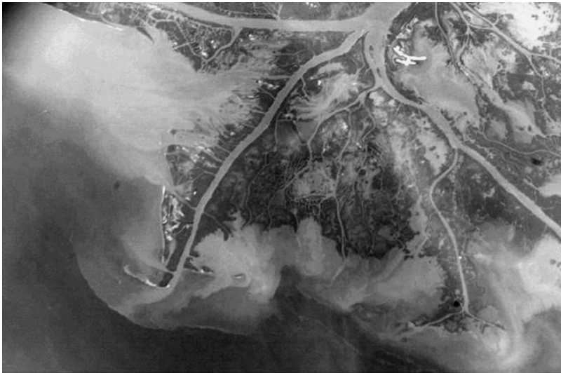
Figure 8.3. Deposition of sediment. Salt water can hold much less sediment than fresh water. Thus mud flowing from the Mississippi is deposited in the Gulf of Mexico in an alluvial plain. Modern deposition is quite prominent in this satellite image, and the entire region south of New Orleans has been built in this fashion. Credits: Mississippi delta - http://eol.jsc.nasa.gov/sseop/clickmap/ cite as above image Miss_deltaISS011-E-5949
