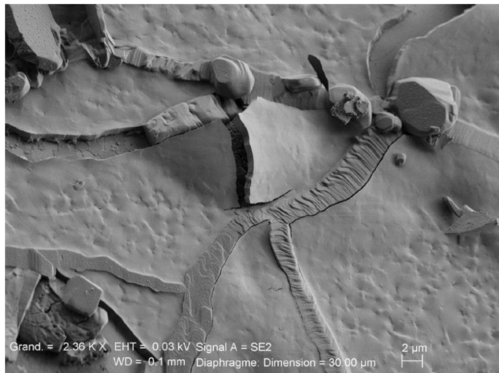
Fig. 11.7 Extremely low landing energy ( E_0=0.030 keV) SEM image of silica ( \text{SiO}_2 ) prepared with an Everhart-Thornley E-T(positive bias) detector and a beam current of 250 pA revealing fine-scale texture and surface topography; Bar = 2 \mu\text{m} (Image courtesy of Carl Zeiss)
