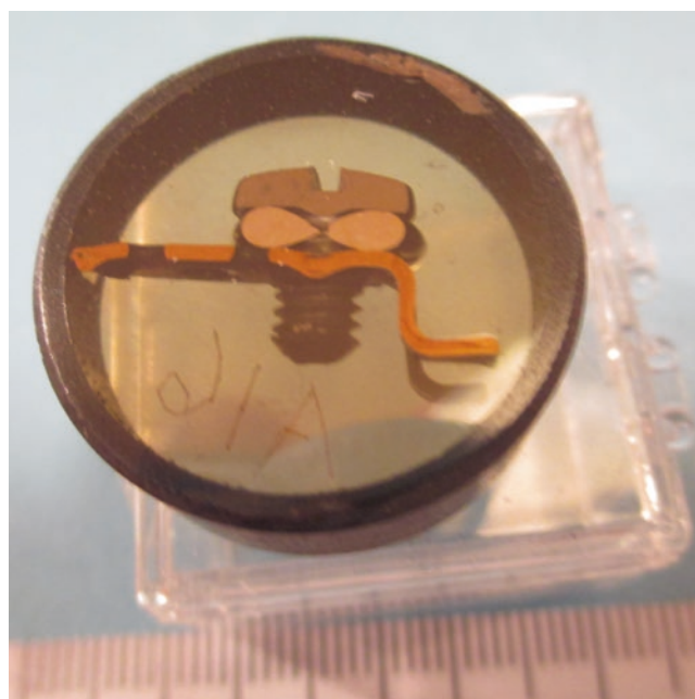
Fig. 27.7 Metallographic mount (2.5-cm diameter) showing the cross section of the steel screw, aluminum wire, and brass plate
