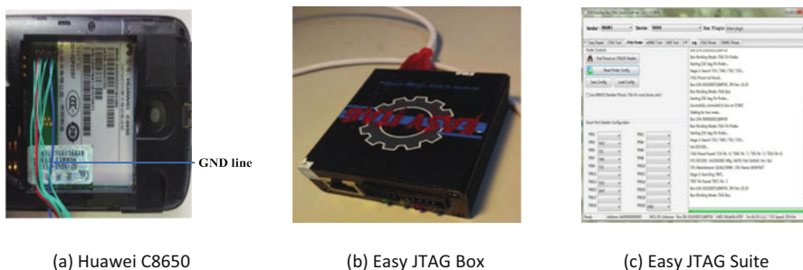
Fig. 15.6 JTAG mobile device imaging. (a) Huawei C8650. (b) Easy JTAG Box. (c) Easy JTAG Suite
