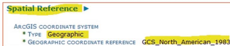
**Note:** lake.tif is projected and GPS.shp is not projected, but both represent the same area. ArcGIS can display both files on the fly.
