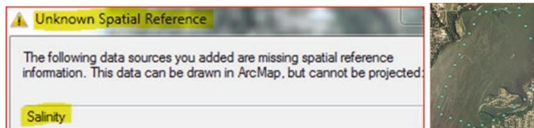
**Result:** The **Salinity.shp** is not displayed in the extent of the **lake.tif** and **GPS.shp**, because the Salinity layer is missing spatial information. This means that the “**Salinity.shp**” is missing the file “**Salinity.prj**.”
