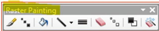
**Note:** The **Raster Painting** toolbar supports **9 tools** designed for drawing and erasing raster cells. In this exercise, we are
