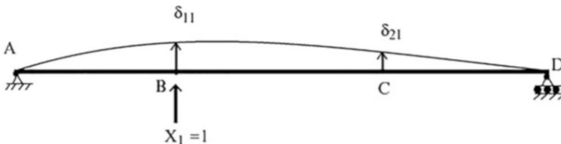
**Fig. E9.3c** Deflected shape due to  $X_1 = 1$
