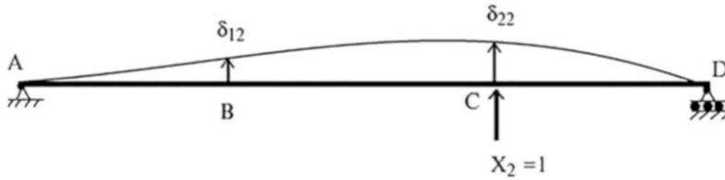
**Fig. E9.3d** Deflected shape due to  $X_2 = 1$
