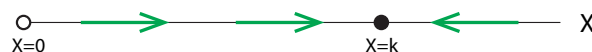
Figure 3.5: A phase portrait of the logistic equation showing unstable (left) and stable (right) equilibria.
