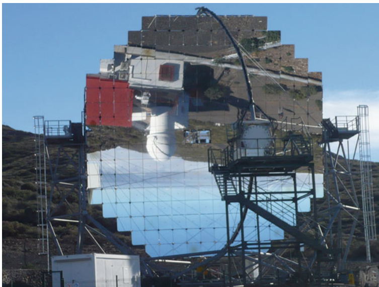
Fig. 1.51 One of the two MAGIC telescopes, located at the Roque de los Muchachos Observatory on La Palma. With their 17 m diameter, the MAGIC telescopes observe the Cherenkov radiation from air showers generated by TeV photons. The detector consists of >450 photo-multipliers
