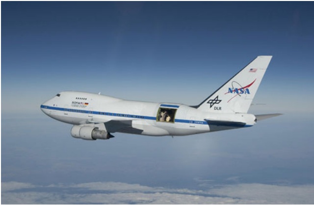
Fig. 1.34 Stratospheric Observatory for Infrared Astronomy (SOFIA), a 2.5-m telescope onboard a refurbished Boeing 747 aircraft, designed to fly at 12 km altitude. A huge door was installed which opens at the high cruising altitude to allow for astronomical observations—a substantial challenge for the structural stability of the aircraft. Regular observations with SOFIA started in 2010. Credit: NASA/Jim Ross
