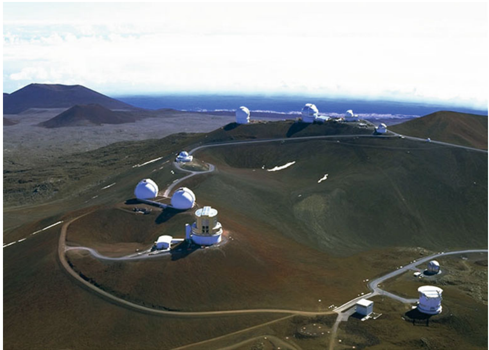
Fig. 1.35 Telescopes at the summit of Mauna Kea, Hawaii, at an altitude of 4200 m. The cylindrical dome to the left and below the center of the image contains the Subaru 8-m telescope; just behind it are the two 10-m Keck telescopes. The two large domes at the back house the Canada-France-Hawaii telescope (CFHT, 3.6 m) and the 8-m Gemini North. The telescope at the lower right is the 15-m James Clerk Maxwell sub-millimeter telescope (JCMT). Credit: R. Wainscoat, University of Hawaii
