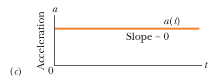
Figure 2-9 (a) The position x(t) of a particle moving with constant acceleration. (b) Its velocity v(t) , given at each point by the slope of the curve of x(t) . (c) Its (constant) acceleration, equal to the (constant) slope of the curve of v(t) .
