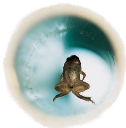
Figure 32-13 An overhead view of a frog that is being levitated in a magnetic field produced by current in a vertical solenoid below the frog.
