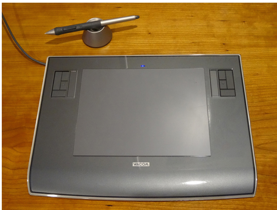
Figure 13.34 A tablet with a specially designed pen to write with is another application of magnetic induction. (credit: Jane Whitney)
