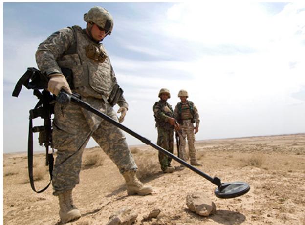
Figure 13.25 A soldier in Iraq uses a metal detector to search for explosives and weapons. (credit: U.S. Army)
