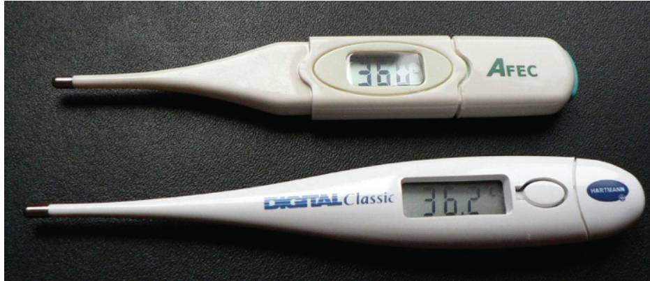
Figure 9.17 These familiar thermometers are based on the automated measurement of a thermistor's temperature-dependent resistance.
