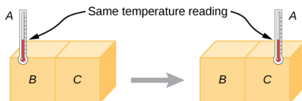
Figure 1.2 If thermometer A is in thermal equilibrium with object B , and B is in thermal equilibrium with C , then A is in thermal equilibrium with C . Therefore, the reading on A stays the same when A is moved over to make contact with C .
