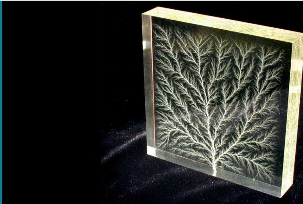
Figure 8.1 The tree-like branch patterns in this clear Plexiglas® block are known as a Lichtenberg figure, named for the German physicist Georg Christof Lichtenberg (1742–1799), who was the first to study these patterns. The “branches” are created by the dielectric breakdown produced by a strong electric field. (credit: modification of work by Bert Hickman)
