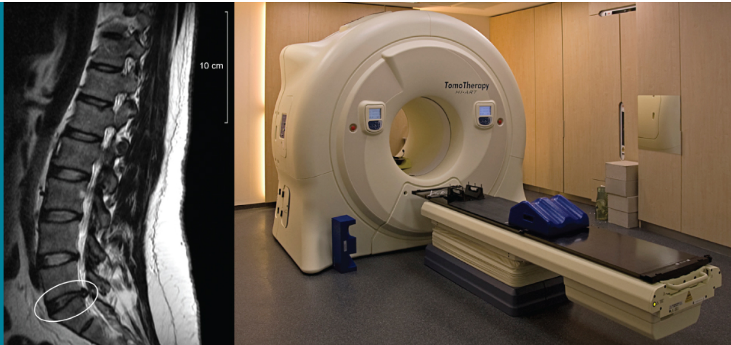
Figure 9.1 Magnetic resonance imaging (MRI) uses superconducting magnets and produces high-resolution images without the danger of radiation. The image on the left shows the spacing of vertebrae along a human spinal column, with the circle indicating where the vertebrae are too close due to a ruptured disc. On the right is a picture of the MRI instrument, which surrounds the patient on all sides. A large amount of electrical current is required to operate the electromagnets (credit right: modification of work by “digital cat”/Flickr).
