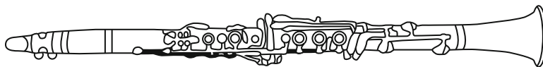
Fig. 24.1 The clarinet resembles a cylindrical pipe, open at one end and closed at the other
