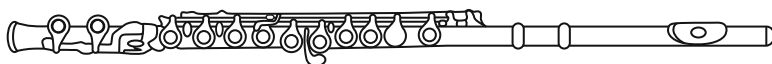
Fig. 24.8 The flute looks complicated, but it is basically a cylindrical pipe with holes in the wall
